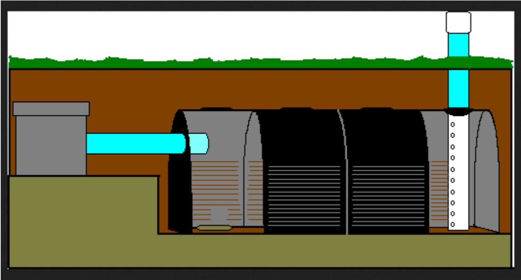
Backfilling the system is recommended without driving over the trenches-mound the dirt slightly over each chamber to account for settling. A track skid steer may be utilized for back filling, but no hard tire equipment which could damage the chambers.
