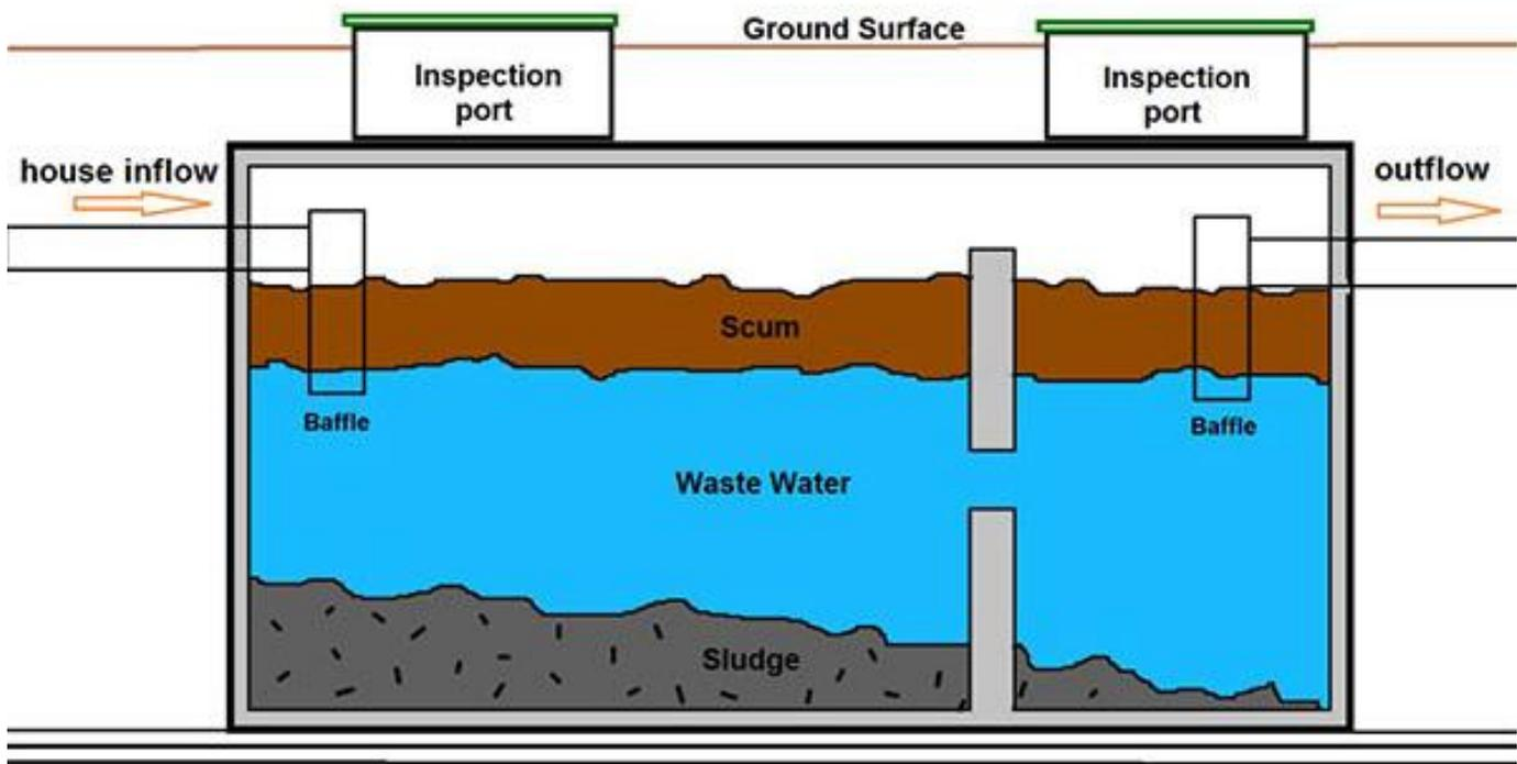
Pipe from the home to the tank and from the tank to the header must be 1% slope (1" drop per 8') and be schedule 40 type pipe
